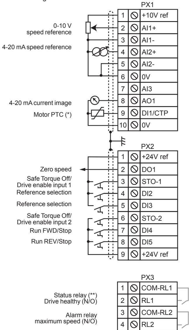
• **Modification of the Run/Stop control logic**
