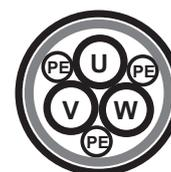
Example: Cable cross-section of 2 x [3 x 150 + PE] corresponds to 2 cables each consisting of 3 phase conductors (cross-section 150 mm<sup>2</sup>) + earth conductors (see below).
