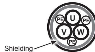
A separate PE protective conductor is mandatory if the conductivity of the cable shielding is less than 50% of the conductivity of the phase conductor.
