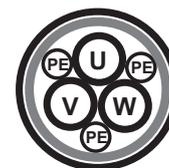
(4) The earth (PE) conductor cross-section cannot be less than half the cross-section of a live conductor, with the same material used. Example: The earth conductor cross-section for a live conductor 2x 240 mm<sup>2</sup> must be:
