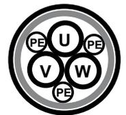
(4) The earth (PE) conductor cross-section cannot be less than half the cross-section of a live conductor, with the same material used. Example: The earth conductor cross-section for a live conductor 2x 240 mm<sup>2</sup> must be:
