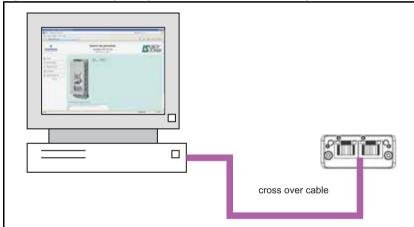
Figure 4-3 Connecting a single PC to MDX-ETHERNET using a crossover cable
