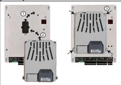
First, remove the mask which protects the option connector slot on the drive control board (1). The option module connector is located on the underside of the module. Push this into the option module slot located on the drive until it clicks into place (2). Screw the module to secure it onto the drive (3).
