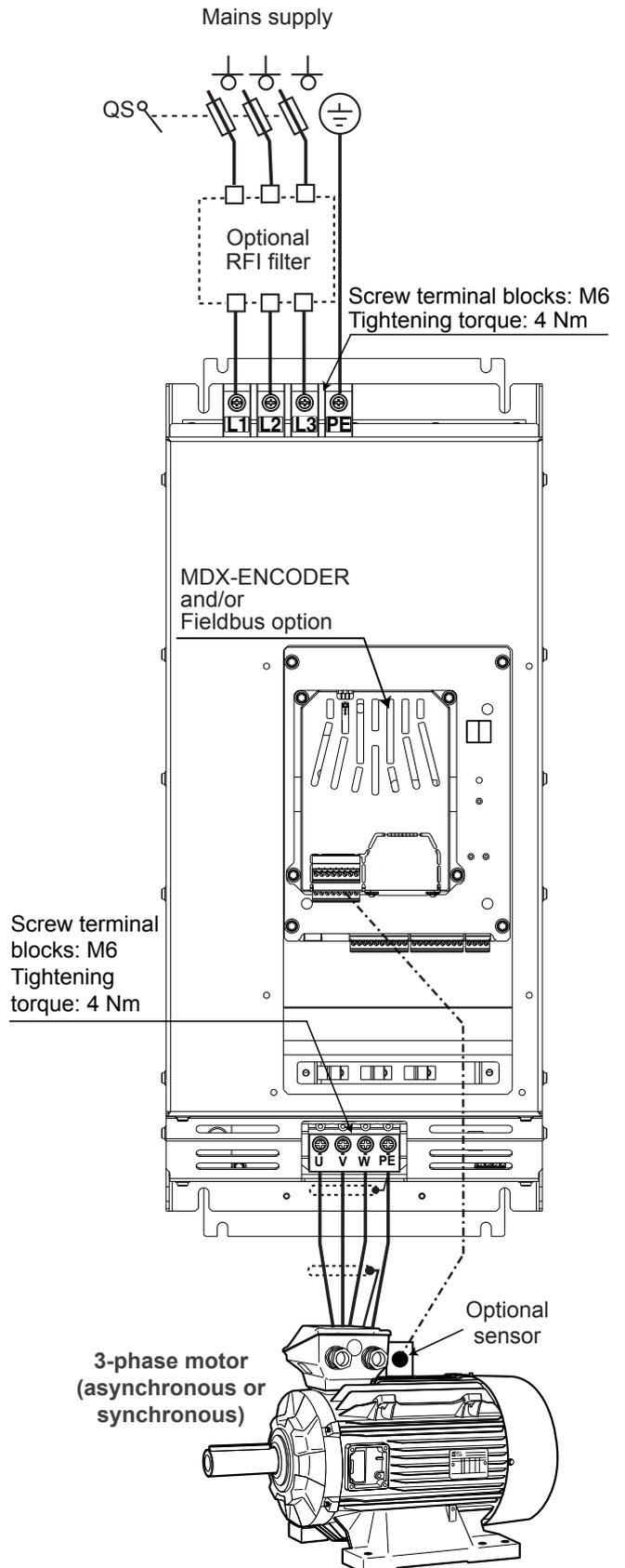
QS: Fused isolator. QS must be opened before working on any electrical parts of the drive or motor.
