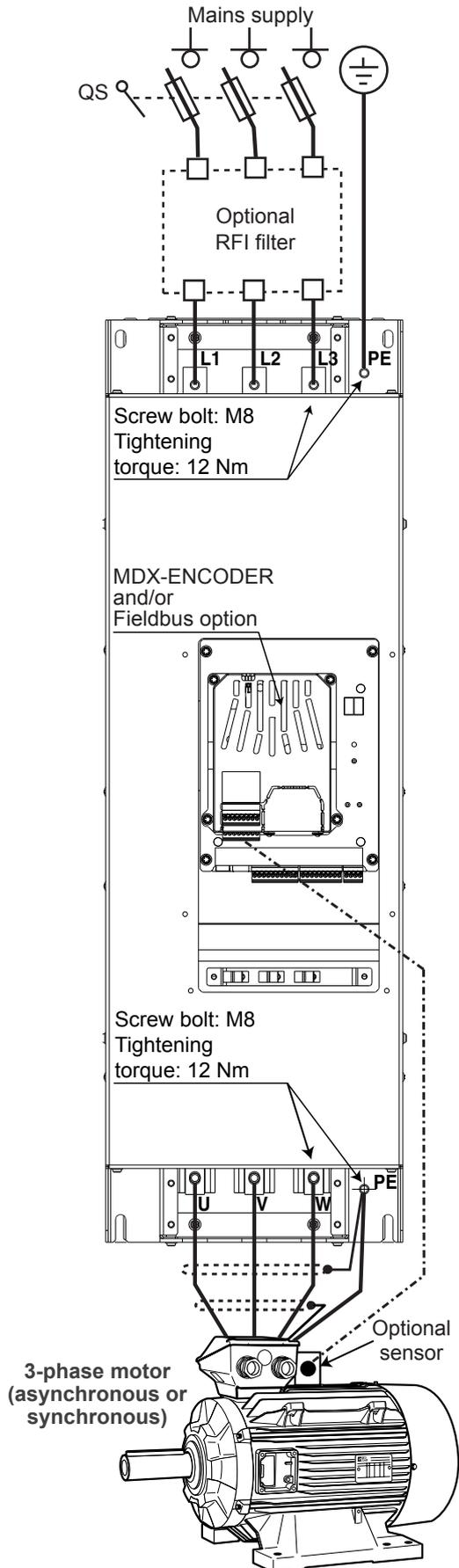
QS: Fused isolator. QS must be opened before working on any electrical parts of the drive or motor.
