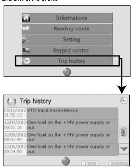
When the drive trips, it is displayed in a red banner, at the top of the interface screen. When the drive trips an alarm, it is displayed in a orange banner.
