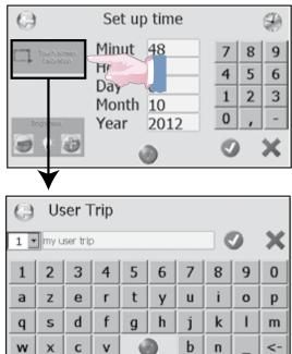
1 Select the trip number to be modified, then 2 use the keypad to type the text, then 3 confirm.
