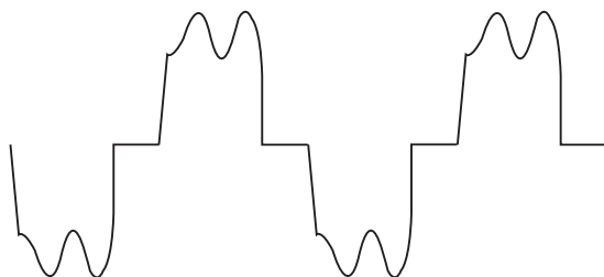
3-phase rectifier line current consumption.
